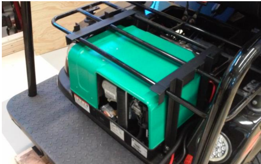
Figure 11. Photograph of generator mount.
